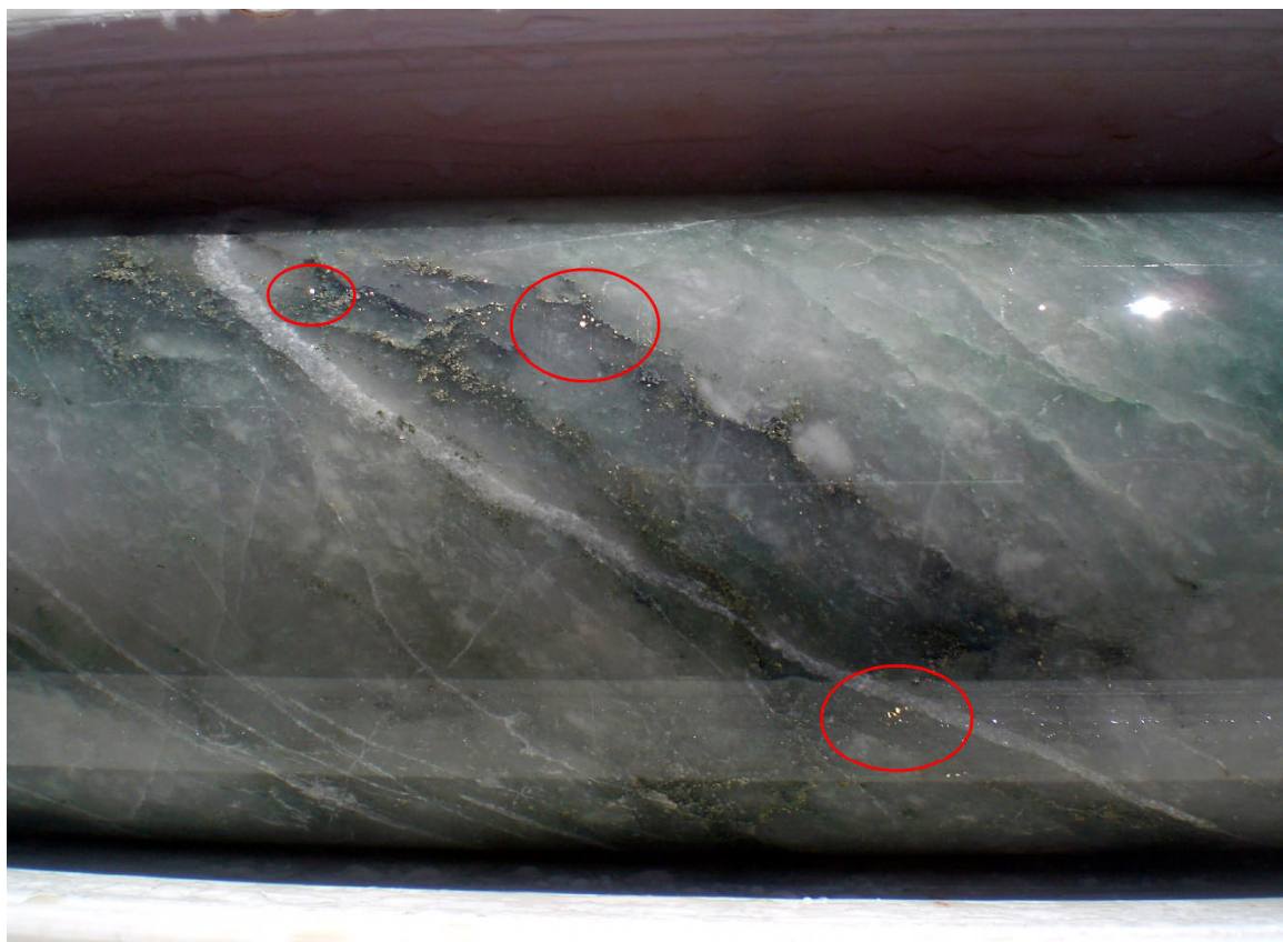
Figure Two: HQ drill core from hole MNDD011 showing intercept through the Wilber Lode at 163.8m to 166.8m down hole depth. Core diameter is 63.5mm.
